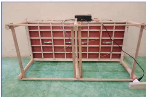
FIGURE 7. Installing the Detector on a Miniature Bridge
